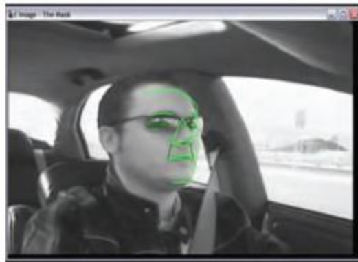
Figure 9. Computer-Based Algorithm Tracking Subtle Changes in Driver Behavior (Campbell, 2012)
